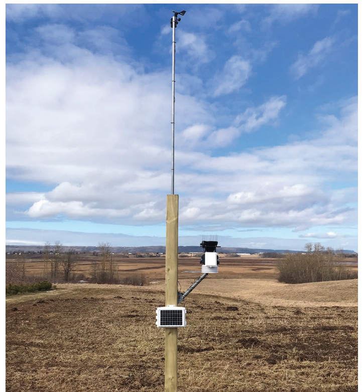
Automated weather stations can be used to record temperature data for growing degree day calculations.
